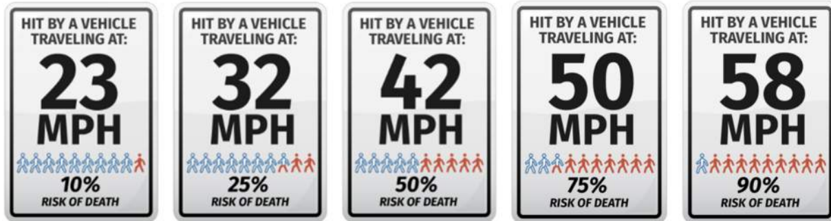
Figure 57. Increased Risk of Death by Speed, Source: USDOT Pedestrian Safety Action Plan
