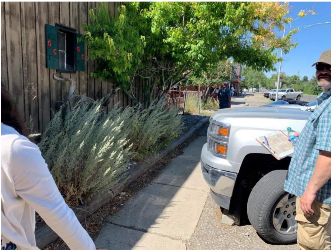
Figure 14. Along 14th Street, head-in parking overhangs the wheel stops and encroaches onto the narrow sidewalk leaving very little space for people to walk. A quick fix to this scenario would be to move the wheel stops back a foot.
